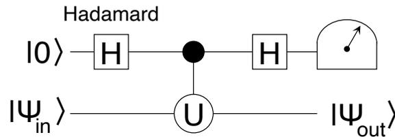
The above two-qubit circuit contains a pair of Hadamard gates (H) acting on the first qubit and a controlled- $U$  operation, meaning that the operator  $U$  acts on the second qubit if and only if the first qubit is in the state  $|1\rangle$ . At the end of the circuit the first qubit is measured.
